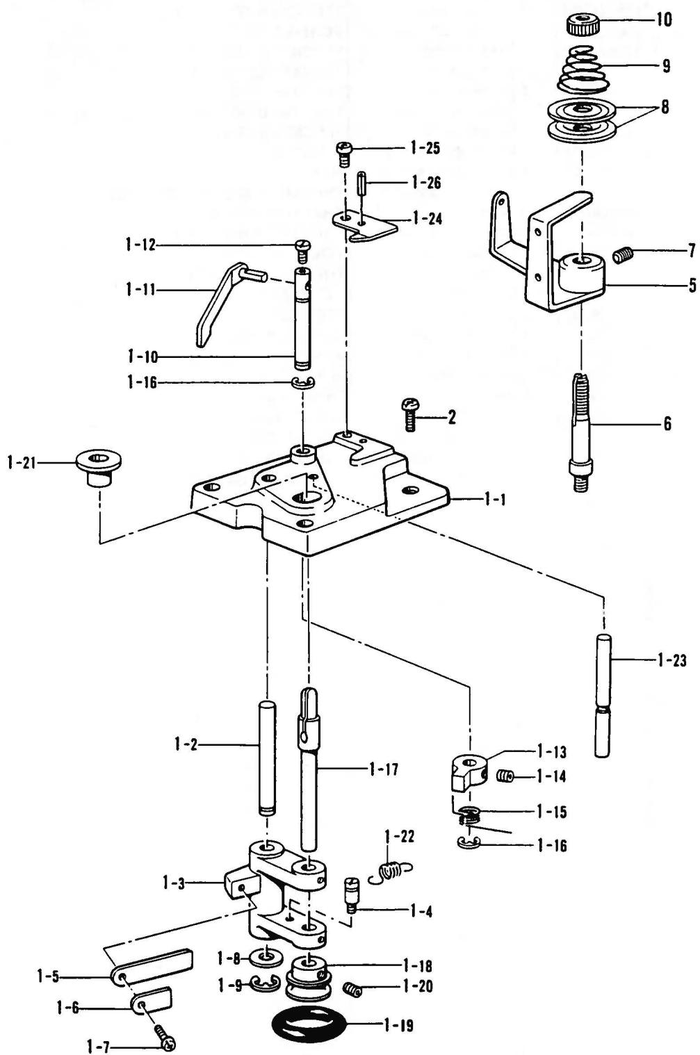
K. 糸巻関係/Bobbin winder mechanism/Spuler/
